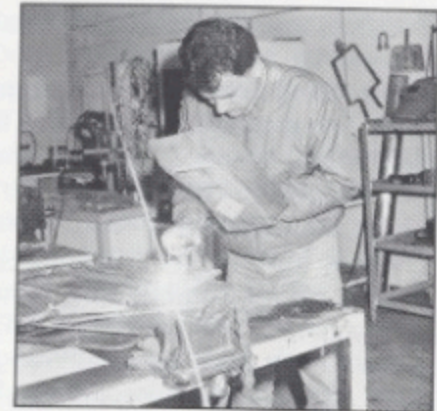
Evgeny Psillouras manufacturing a boiler manifold
