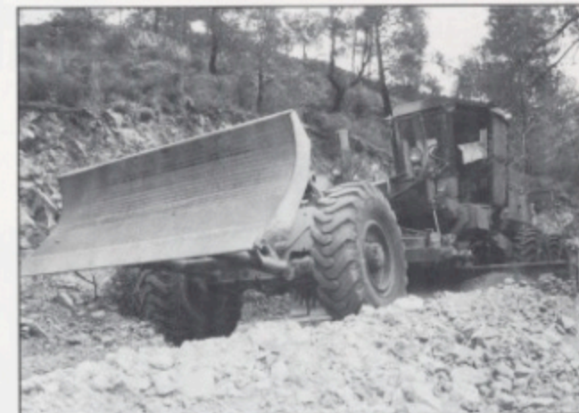
LCpl Simpson operating ASG 113 (Grader) on Western Sector (C Company) of Sector One (DANCON)
