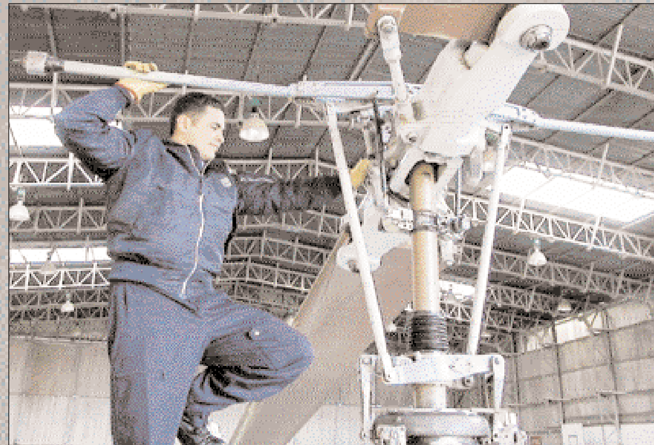
Before take off, Sergeant Gustavo Filippini inspects the main rotor of the Bell 212
